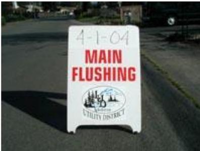
Lakehaven Utility District is working to clean its entire water main system through a program called Systematic Flushing. District crews have been working in street intersections and at the end of cul-de-sacs opening and operating fire hydrants and blow-offs to create high water flows and velocities in the water system to scour and clean the inside of our water mains. Letters are mailed a week in advance notifying
